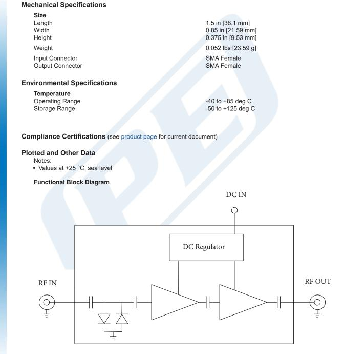
Click the following link (or enter part number in "SEARCH" on website) to obtain additional part information including price, inventory and certifications: 1.2 dB NF Input Protected Low Noise Amplifier, Operating from 1 GHz to 1.4 GHz with 30 dB Gain, 10 dBm P1dB and SMA PE15A63006
