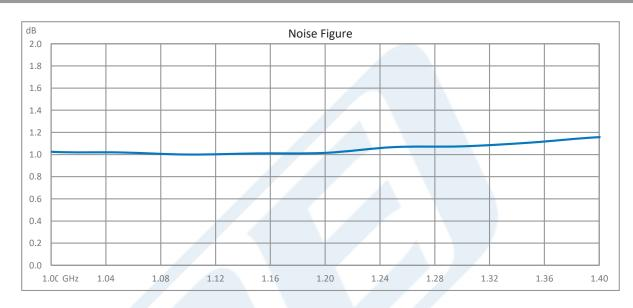
1.2 dB NF Input Protected Low Noise Amplifier, Operating from 1 GHz to 1.4 GHz with 30 dB Gain, 10 dBm P1dB and SMA from Pasternack Enterprises has same day shipment for domestic and International orders. Our RF, microwave and millimeter wave products maintain a 99.4% availability and are part of the broadest selection in the industry.
