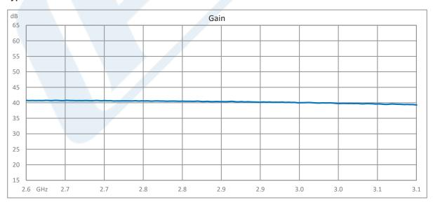
Click the following link (or enter part number in "SEARCH" on website) to obtain additional part information including price, inventory and certifications: 1.2 dB NF Input Protected Low Noise Amplifier, Operating from 2.6 GHz to 3.1 GHz with 40 dB Gain, 10 dBm P1dB and SMA PE15A63009
