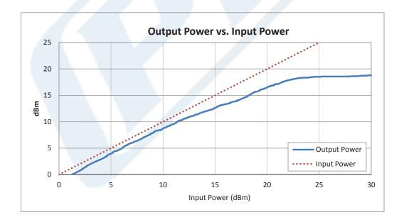
Click the following link (or enter part number in "SEARCH" on website) to obtain additional part information including price, inventory and certifications: High Power Limiter, SMA, 100W Peak Power, 20 ns Recovery, 16 dBm Flat Leakage, 11 GHz to 18 GHz PE8027
